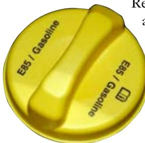
Flexifuel cars are capable on running on E85, petrol only, or any mix of both. (Photo: General Motors)
