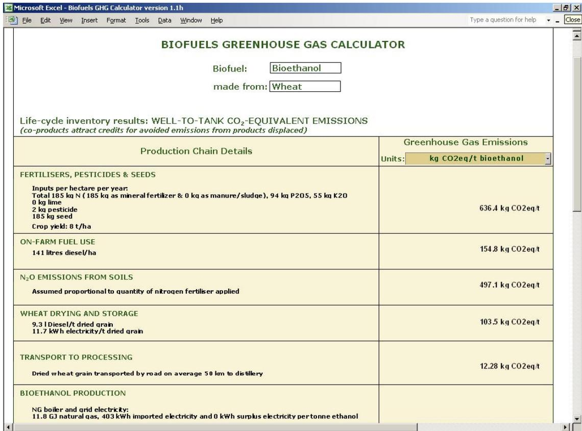
Figure 5: Biofuels Greenhouse Gas Calculator - bioethanol results page
